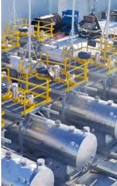
Shop Fabricated Tank Section
