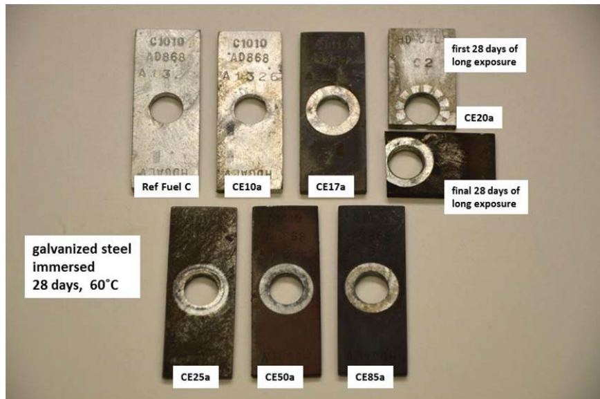
Modest corrosion E85
