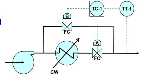
Common Temperature Control System (control station block and bypass valves removed)
