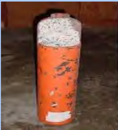
✓ Acetylene Cylinders are filled with Calcium Silicate
