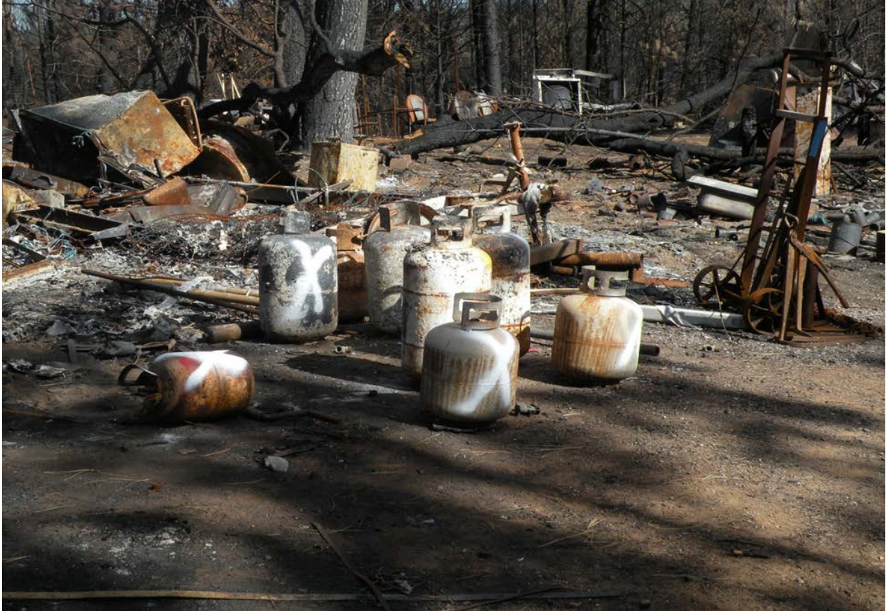
Miscellaneous Tanks De-headed and Marked with a White "X". (Butte Fire - Calaveras County - 2015)
