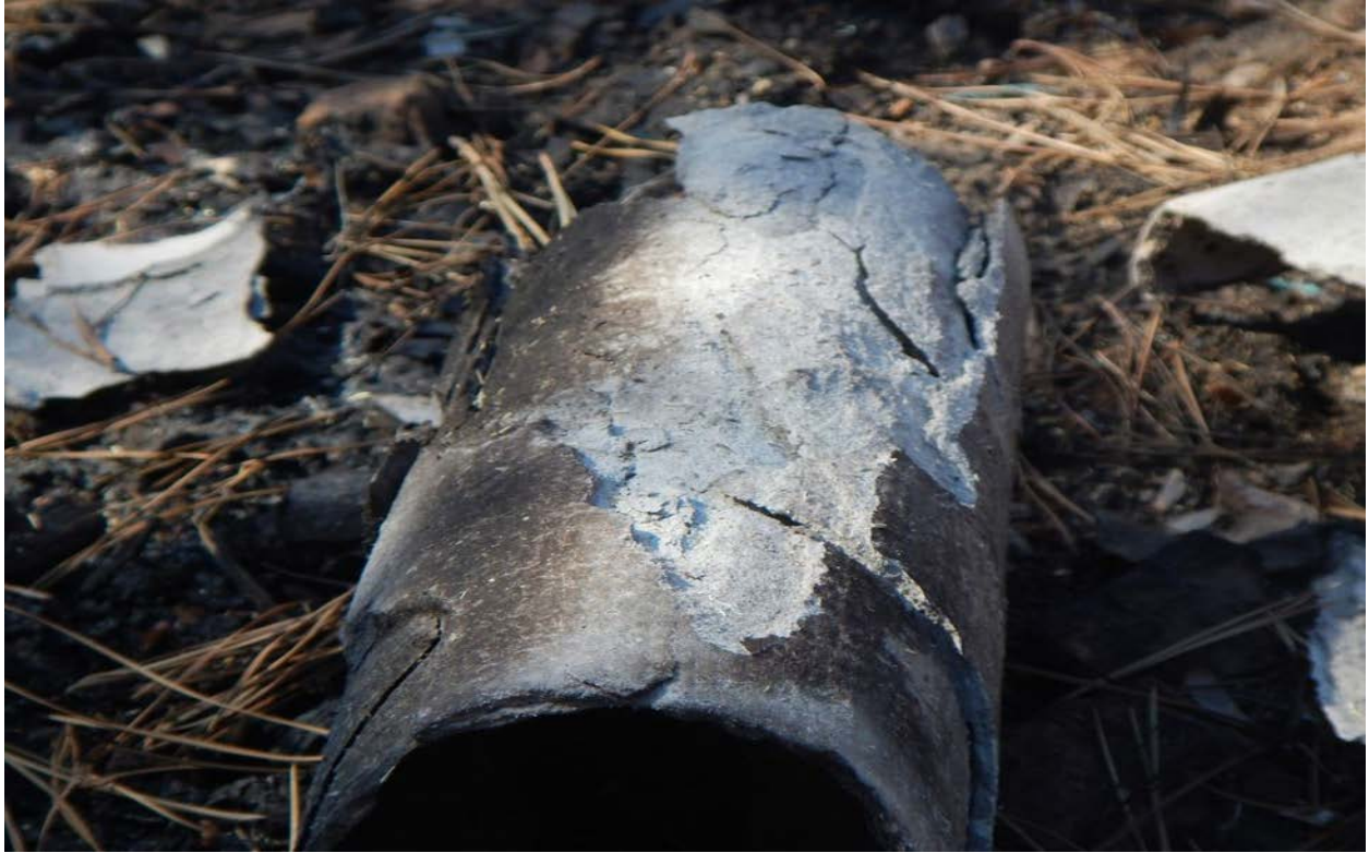
Transite Pipe (Asbestos-Containing Material). (Thomas Fire - Ventura County - 2017)
